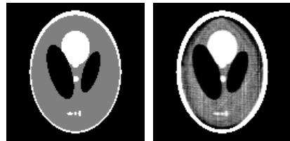
Fig. 1. A slice from a voxelization of the phantom (left) and the corresponding slice obtained from a reconstruction (right). A very narrow display window was chosen to emphasize their difference.
